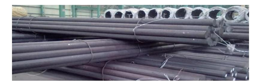
Carbon steel rod is an alloy rod containing carbon and iron, with a carbon content up to 2.1% by weight. Carbon steel bars have good hardness and strength properties and they are cheaper than other steels.
