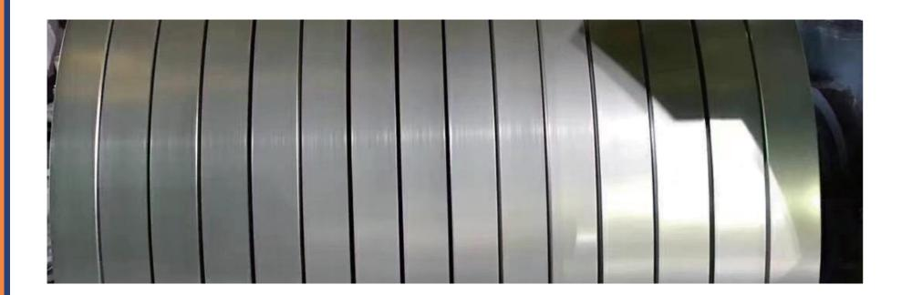
Galvanized steel is defined as a carbon steel sheet coated with zinc on both sides. Zinc coating is one of the most effective and economical method of protecting bare steel from a corroding environment.
