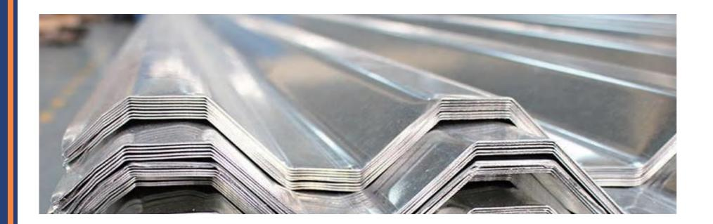
Corrugated sheet is also called profiled sheet, which is made of color coated steel sheet, galvanized sheet and other metal sheets by rolling and cold bending into various wave profiled sheets.
