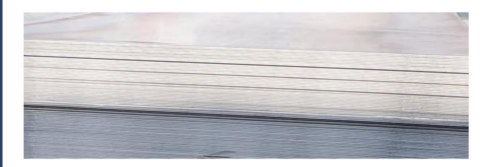
Hot-rolled plate/coil is made by continuously rolling the slab, after heating the slab in the reheating furnace, by the roughing mill and finishing mill, and it is coiled for a easier transportation.
