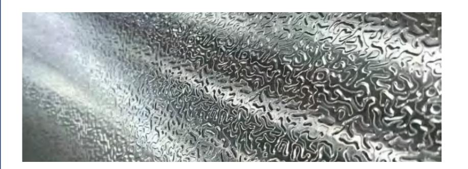
Aluminium embossed sheet is a kind of aluminum product which form a variety of decorative patterns on the surface after rolling process on the basis of the aluminum sheet.
